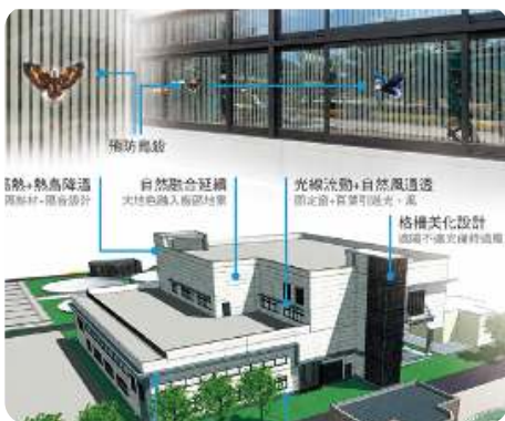
Bird Collision Prevention Window Design Project
