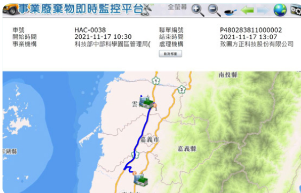
GPS vehicle track record for sludge removal and transportation of sewage to treatment plant (Huwei)
