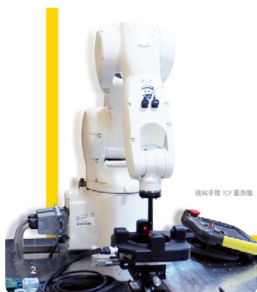
Mechanical Arm Tool Central Point Measuring Instrument
