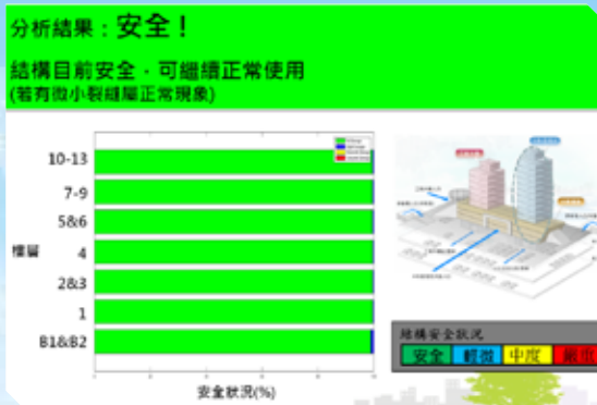
The Structural Safety Monitoring System can provide fast structural health diagnosis and safety assessment after an earthquake occurs
